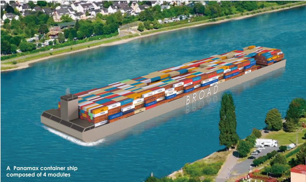
A Panamax container ship composed of 4 modules
